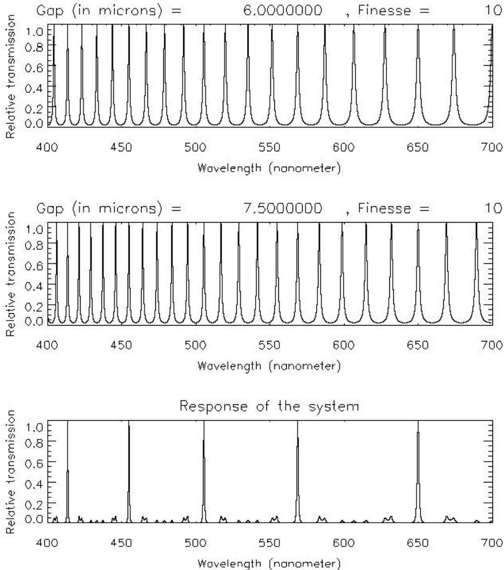
Figure 9: Model response of a twin-etalon system that provides the largest FSR in the visible.
