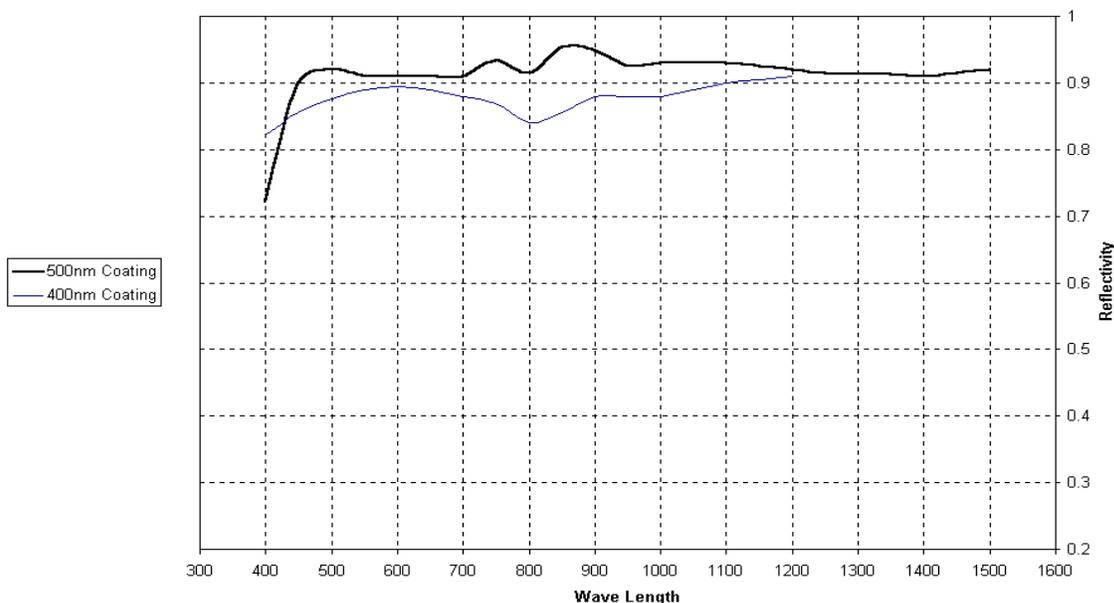
Figure 3: Broadband reflective coatings developed by SSI for the LCFP. Note that the 400nm coating actually extends to 1600nm.
