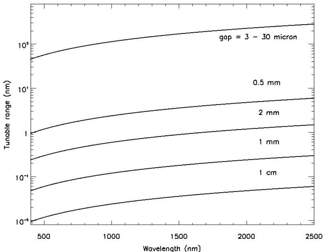
Figure 7: LCFP tunable range as a function of wavelength for different gap sizes.
