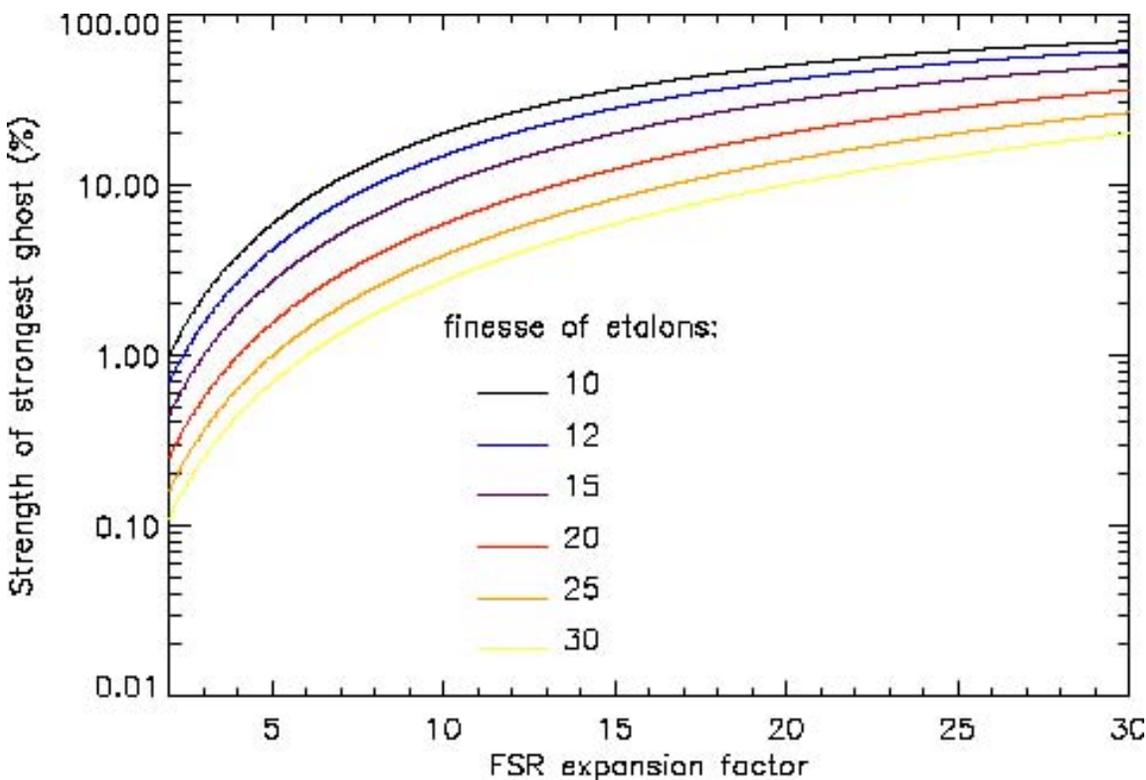
Figure 6: Strength of the strongest ghost relative to the maximum transmission peak as a function of FSR expansion factor and finesse of the etalons for a twin etalon system.
