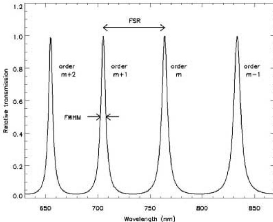
Figure 2: Relative model transmission response of an etalon with a 3  $\mu\text{m}$ -wide gap.
