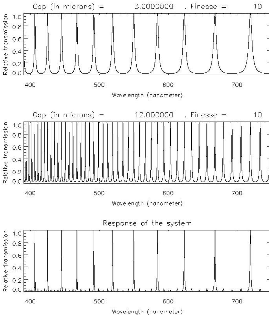
Figure 5: Model illustrative of a two-etalon system.
