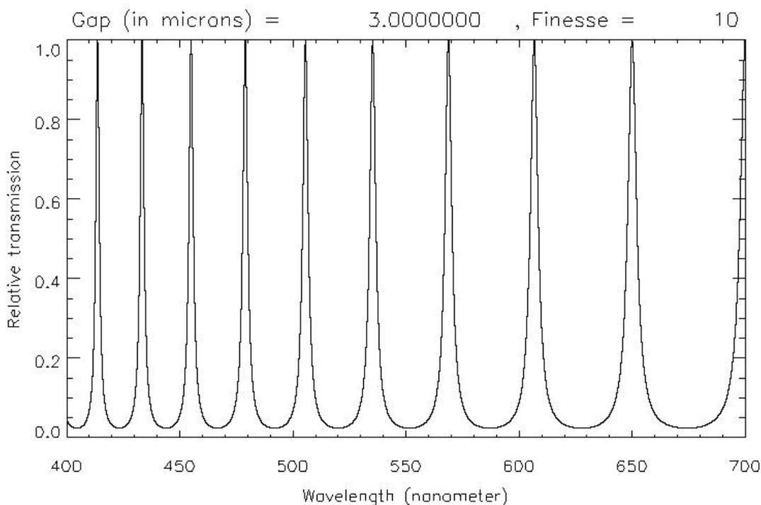
Figure 8: Model of a single-etalon device with a gap size of 3 micron.
