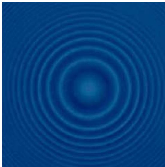
Figure 1: Interference pattern produced by a Fabry-Perot with monochromatic light.
