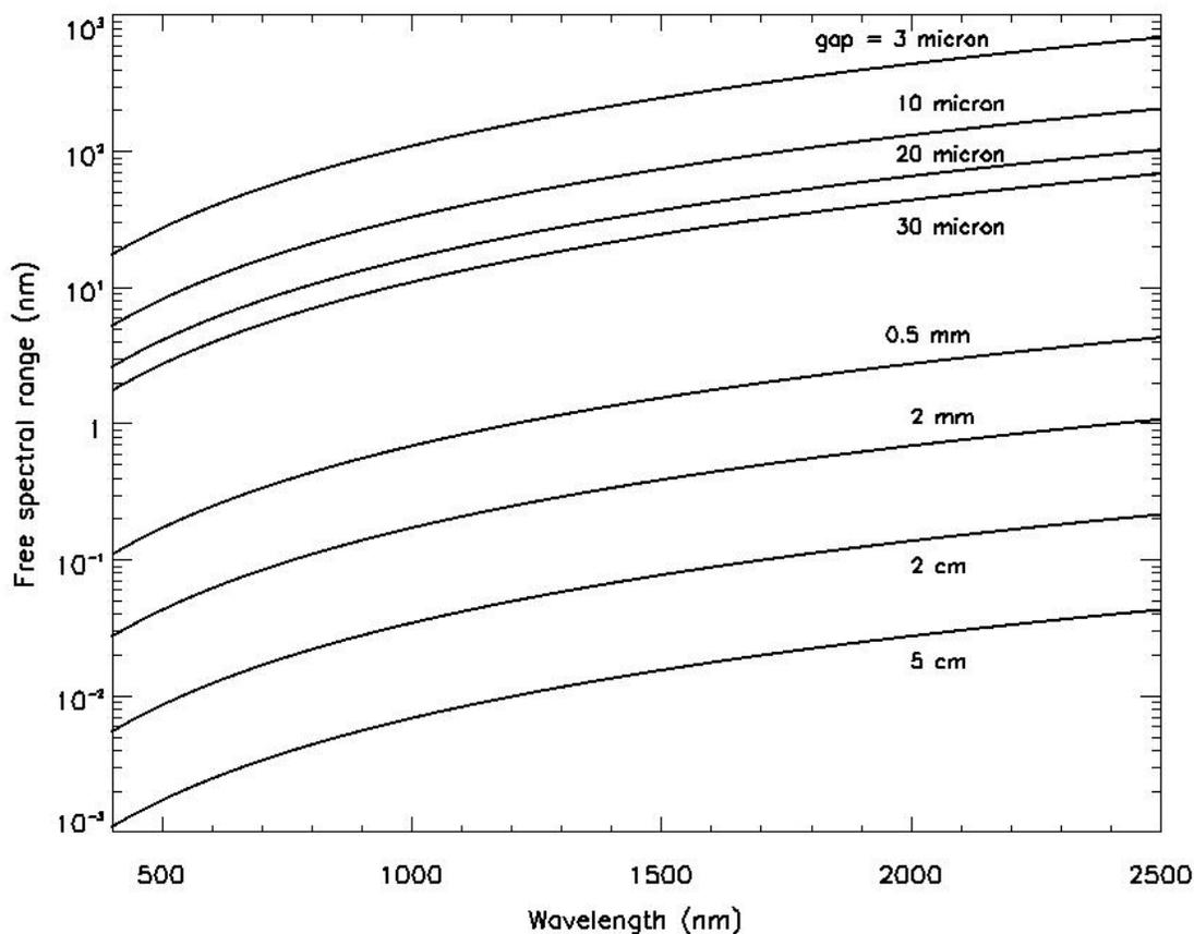
Figure 4: Free Spectral Range as a function of wavelength for one etalon with different gaps.
